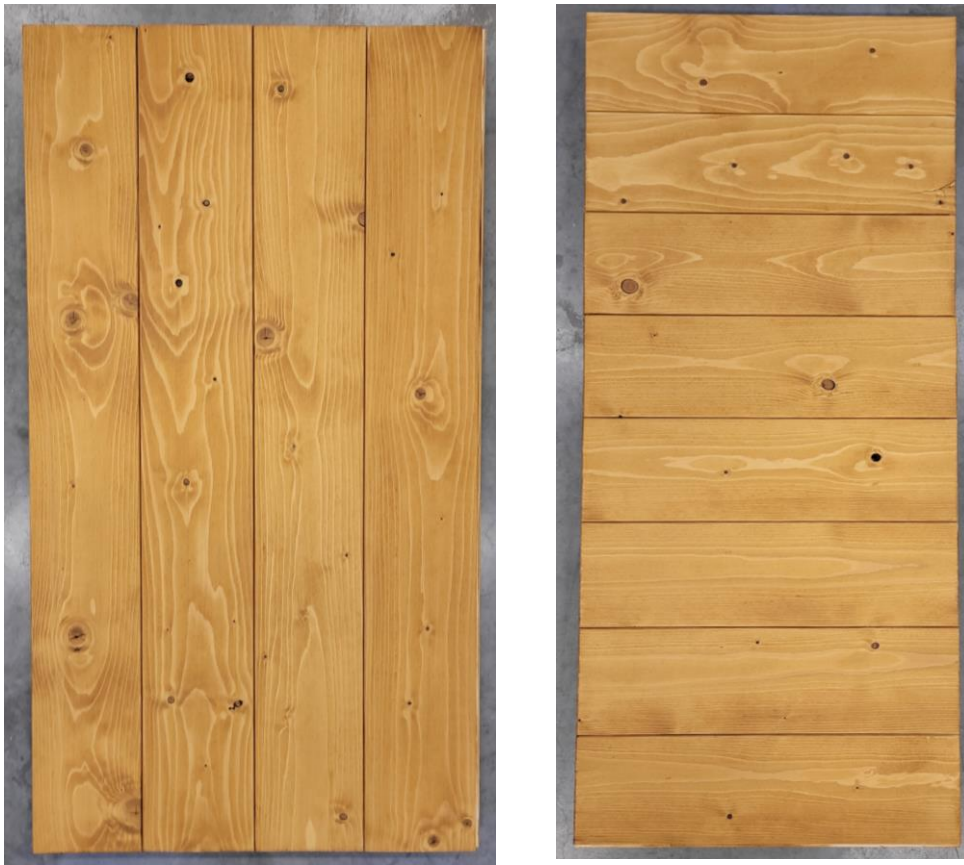
Spruce wood flooring, sanded with grain P80 and coated with Rubio Monocoat DuroGrit (left: longitudinal direction, right: transverse direction)
