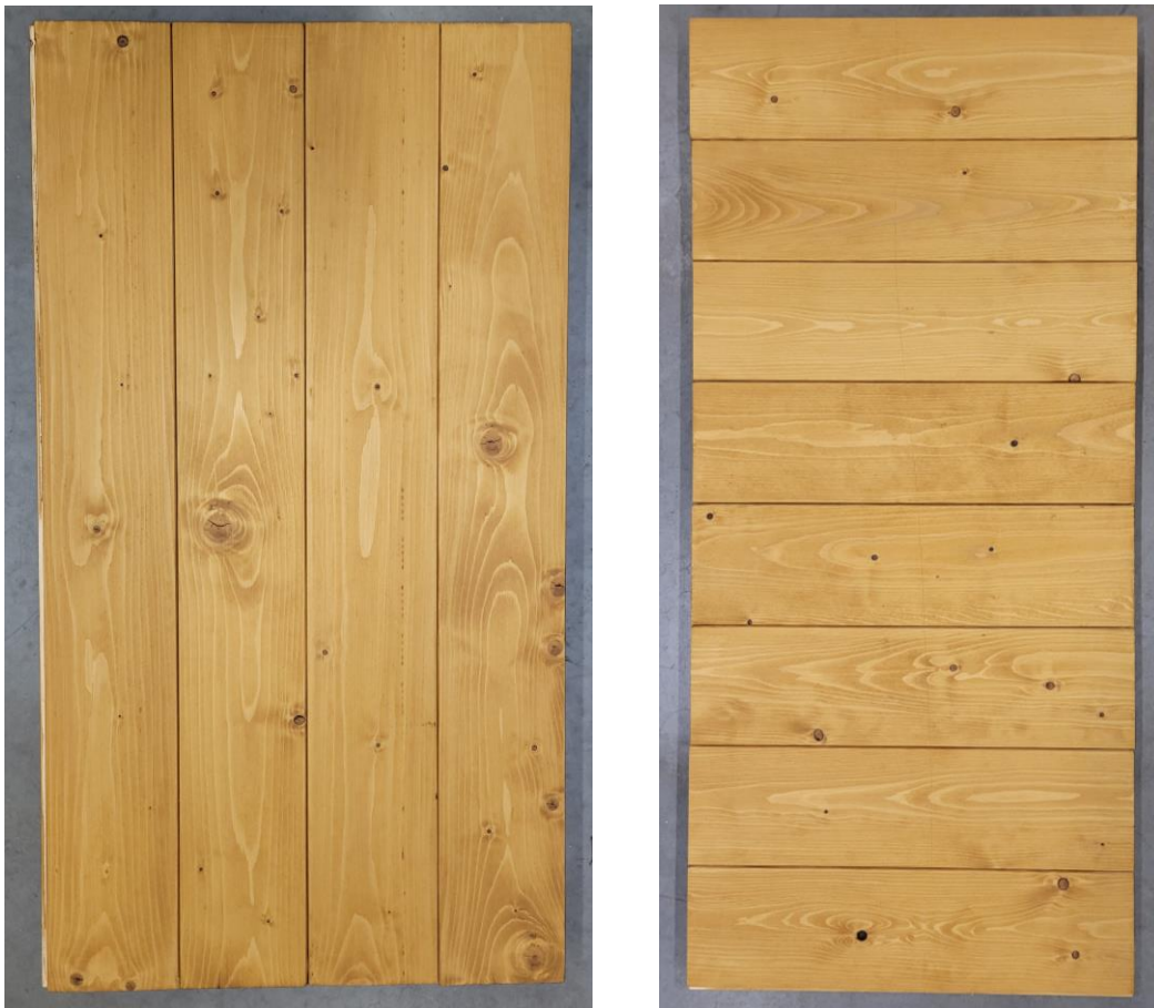
Spruce wood flooring, sanded with grain P120 and coated with Rubio Monocoat DuroGrit (left: longitudinal direction, right: transverse direction)
