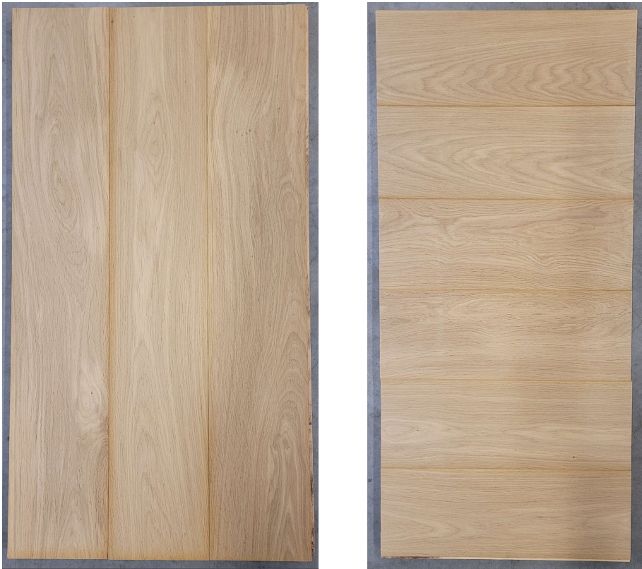
Oak wood flooring, sanded with grain P100 and coated with Rubio Invisible Protector (left: longitudinal direction, right: transverse direction)
